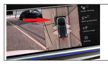
The arrow identifies the line which is shown as not parallel or straight alongside the vehicle.
