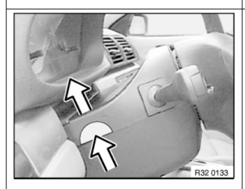
6. Remove the steering column top panel.
