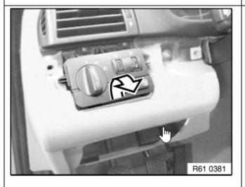
4. Remove the light switch assembly.
