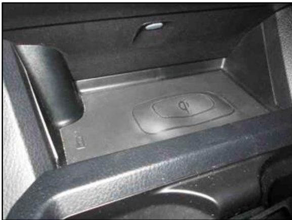
Figure 1. Example of a Deformed Wireless Phone Charger Assembly Rubber Pad
