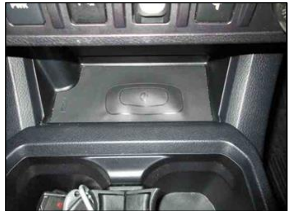
Figure 2. Example of a Deformed Wireless Phone Charger Assembly Rubber Pad
