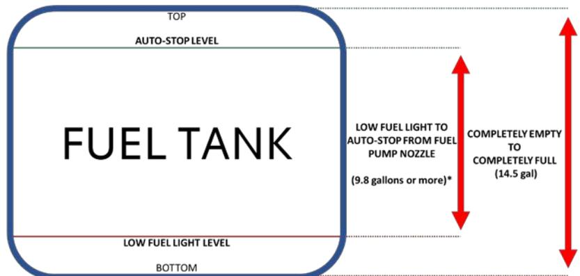
(\*) The refueling amount from low fuel light to auto-stop depends on a number of factors including normal fuel tank production variation, temperature, gas station pump variations, distance travelled since low fuel light illumination and other factors.
