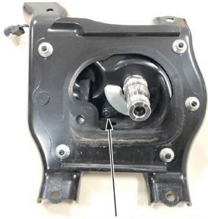
INFRARED TRANSMITTER BOLT Remove. 12 N.m (9 lb-ft)
