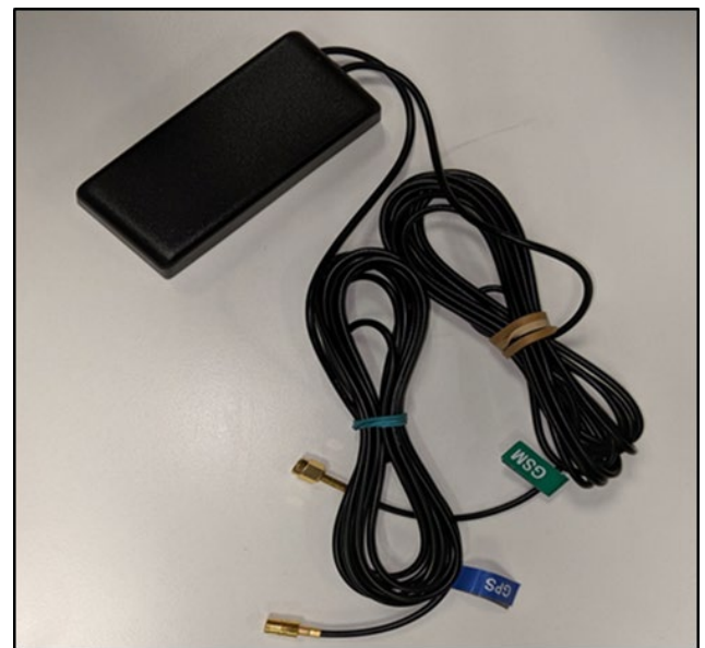
GPS and GPRS antenna
