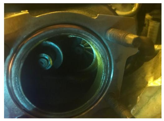
If oil is found at the outlet of the turbocharger on either side, then replace the turbocharger, drive to clean out the exhaust and then let sit to get cold and reevaluate.
