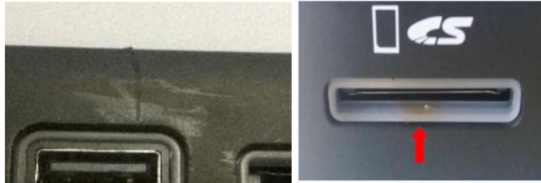
Figure 2: example of cuts or breaks of the plastic frame
