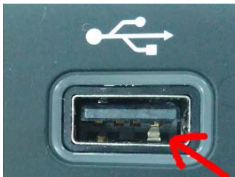
Figure 1: example of Missing or broken Pins
