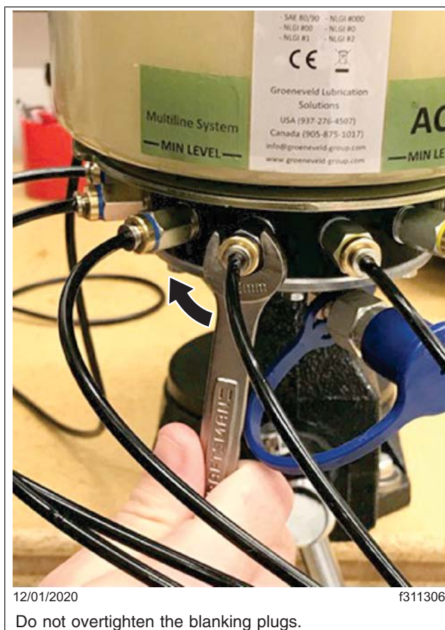
Fig. 1, Tightening the Injectors and Blanking Plugs
