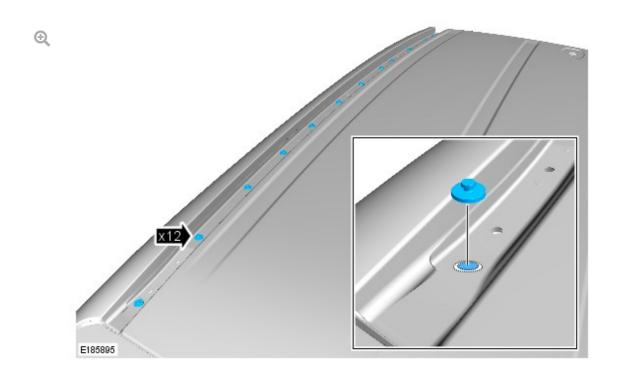
Install the new roof molding studs in the positions previously applied with bonding glue.
