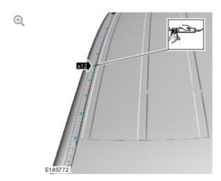
Apply the bonding adhesive to the areas previously marked in Step 4.
