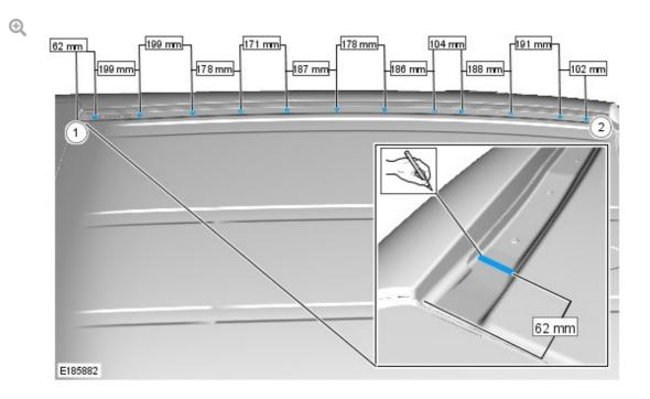
Starting at the windshield (1) and moving towards the rear of the roof panel (2), use a suitable marker to mark the roof channel in the positions indicated.
