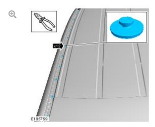
Use a suitable tool to remove the 12 roof molding studs.
