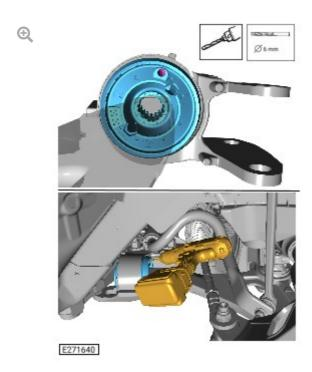
Drill a hole through the rear hydrabush fill port using a 6 mm diameter drill bit, to a depth of no more than 23 mm.
