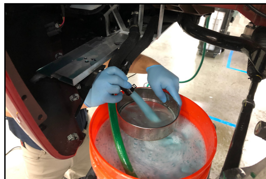
old coolant being collected to be disposed of, screening for debris
