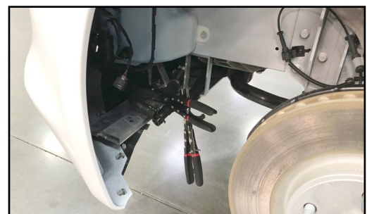
Hose shown clamped before draining.
