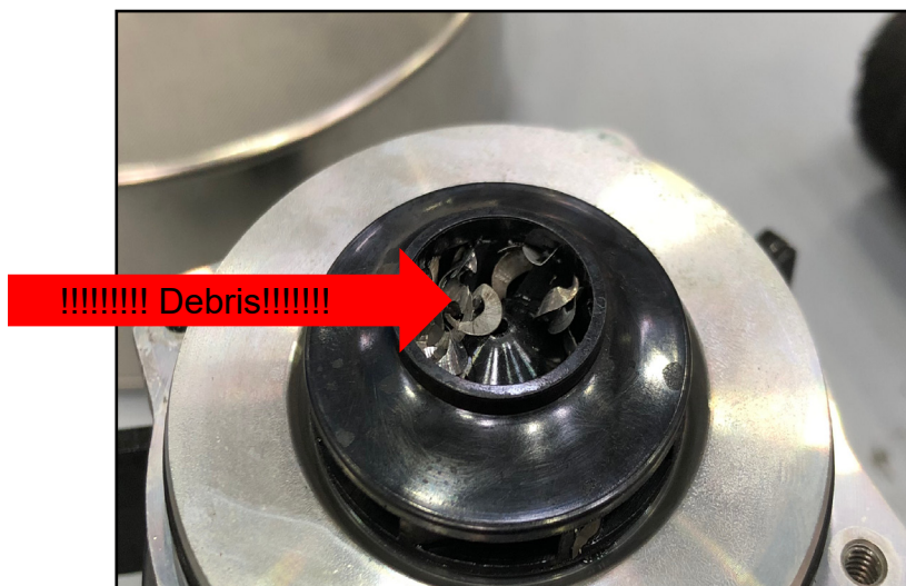
Debris found - replace the pump
