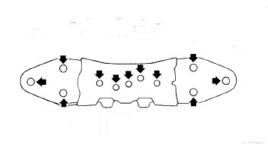
• Lower the transmission stand by **NO MORE THAN 75mm**. Remove the 6 bolts securing the transmission cover then CAREFULLY slide cover toward the rear of the vehicle.
