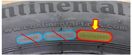
**VERY IMPORTANT:** When performing these inspections, **<u>BOTH</u>** the DOT Serial Number and the Mold Number (circled in **RED, Highlighted and In Parentheses**) must match those provided above. If only one of the 2 numbers match, the tire(s) is not affected.
