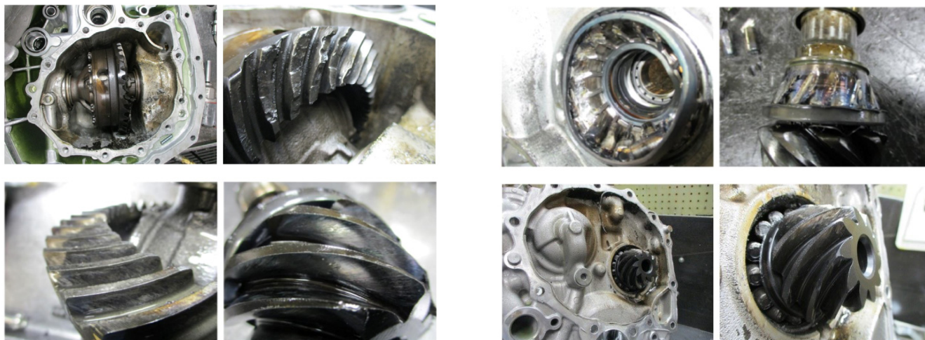
DAMAGED PINION GEAR BEARING ROLLER CAGE
