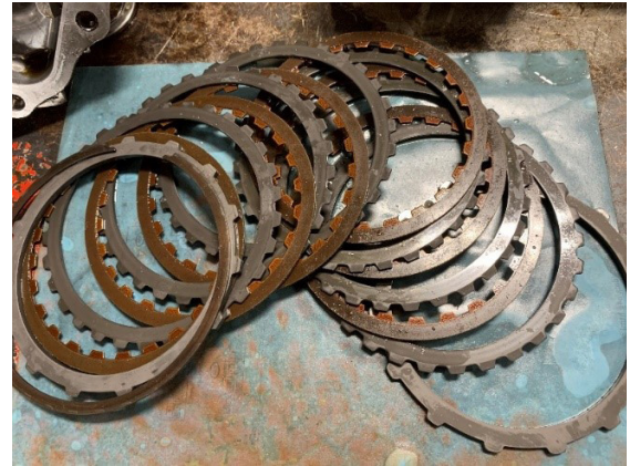
Figure 1: Visually "ok" clutches and plates
