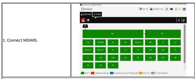
2. Use MDARS to verify if the Telematics Control Unit (TCU) is at the latest software level (Toolbox Software Update Run TCU).
