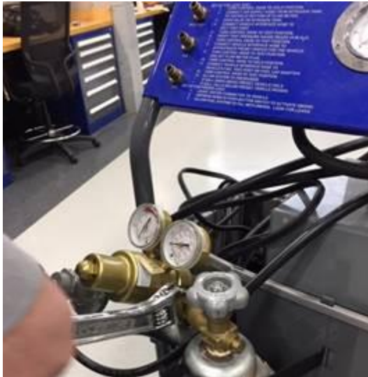
Figure1. Removing the KLI9210DLX manifold.
