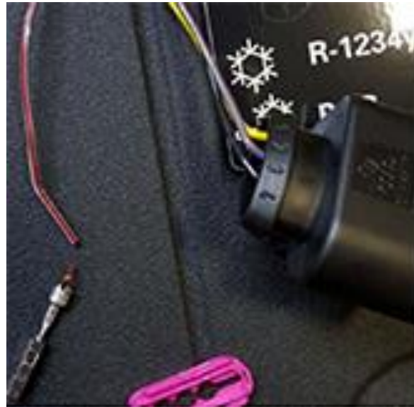
Figure 1. T4e with damaged wire.
