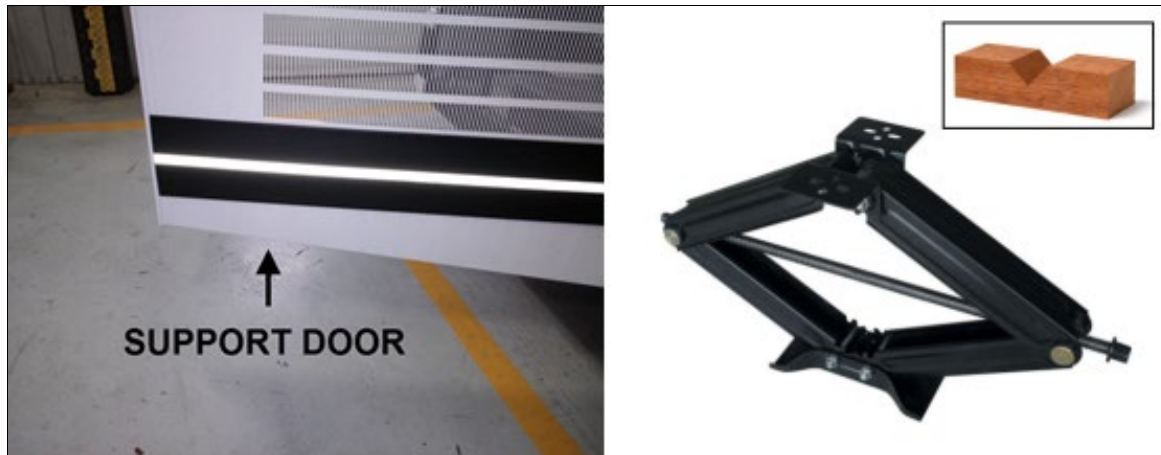
FIGURE 2: SUPPORTING THE DOOR
