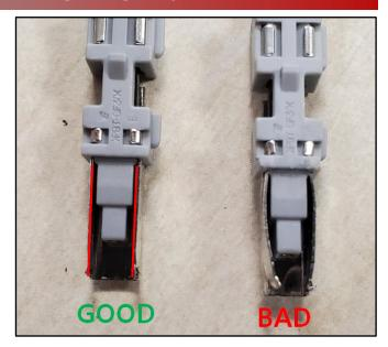
7b. Using needle nose pliers, **gently** squeeze the outer shield on the female terminal to improve the tension. <u>Insert the female pin around the male connector to gauge tension</u>.
