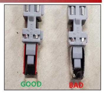
14. Using needle nose pliers, **gently** squeeze the outer shield on the female terminal to improve the tension. Insert the female pin around the male connector to gauge tension.
