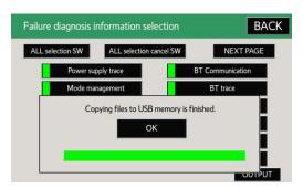
12. Select the "BACK" button in the upper right-hand corner, then turn "Recording ON/OFF" back to the ON position (should be green to enable the MMR to record).
