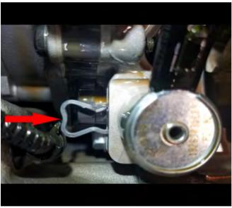
**Important:** Do not use any tools to tap the pressure control valve into place. Only install the pressure control valve by pushing on the body of the valve by hand.
