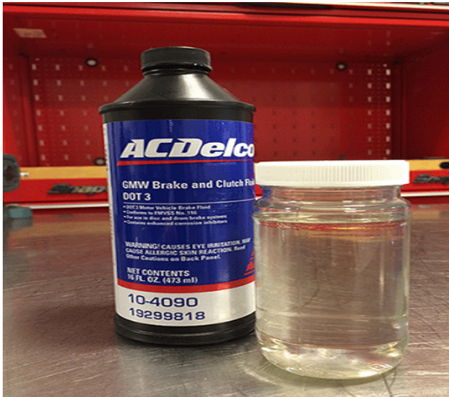
Diesel Exhaust Fluid (DEF) mixed with Brake Fluid.
