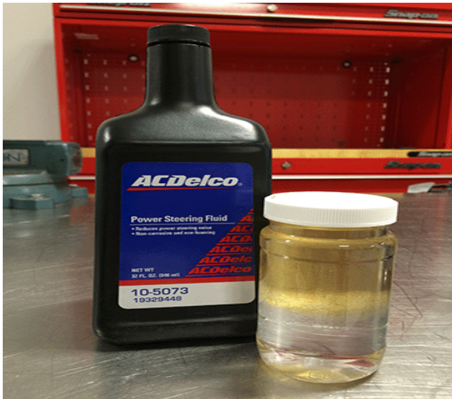
Diesel Exhaust Fluid (DEF) mixed with Power Steering Fluid.
