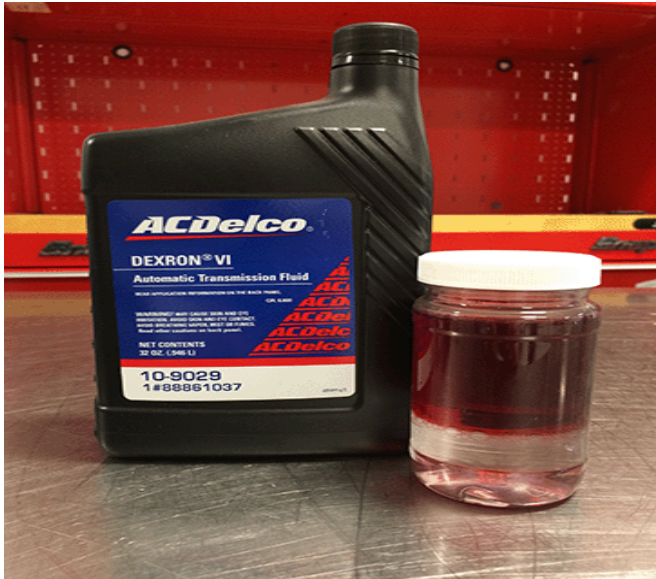
Diesel Exhaust Fluid (DEF) mixed with Power Steering Fluid.
