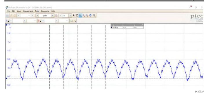
The graphic above depicts an example of a four-cylinder engine with a bad exhaust cam lobe.
