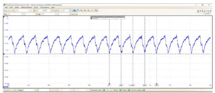
This should help to identify the top of each compression stroke in two rotations of the engine.
