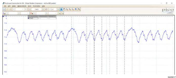
The graphic above depicts an example of an eight-cylinder engine with a cylinder that has no compression in one cylinder.
