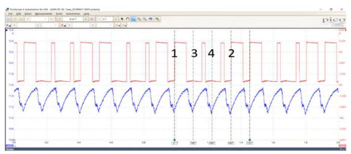
If an engine has low or high compression on one cylinder, it may be useful to add an injector pulse or a Camshaft Position Sensor to help determine which cylinder has an issue.
