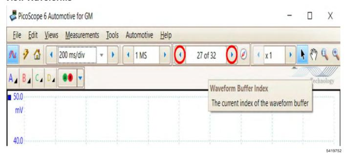
To examine one of these wave forms, use the Waveform Buffer Index navigation buttons to locate the start of the cranking.
