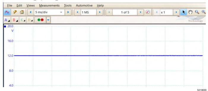
5. With the PioScope hooked up and the software running, a steady line at battery voltage on the graph should be displayed.
