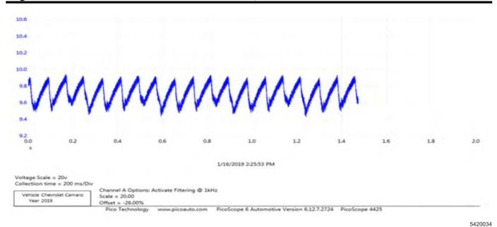
This is a four-cylinder engine with a 40 PSI loss in one cylinder.
