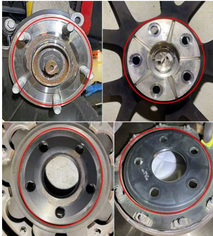
Fig. 1 Areas That Needs To Be Cleaned
