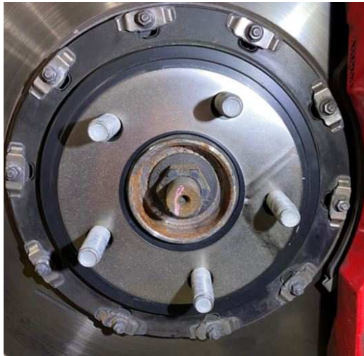
Fig. 4 Friction Disc Installed On The Rotor
