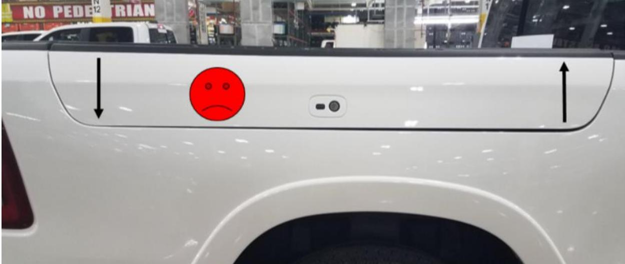
If the gap is higher at the FRONT, open the lid, and apply force to the tool to bend the striker loop rearward.
