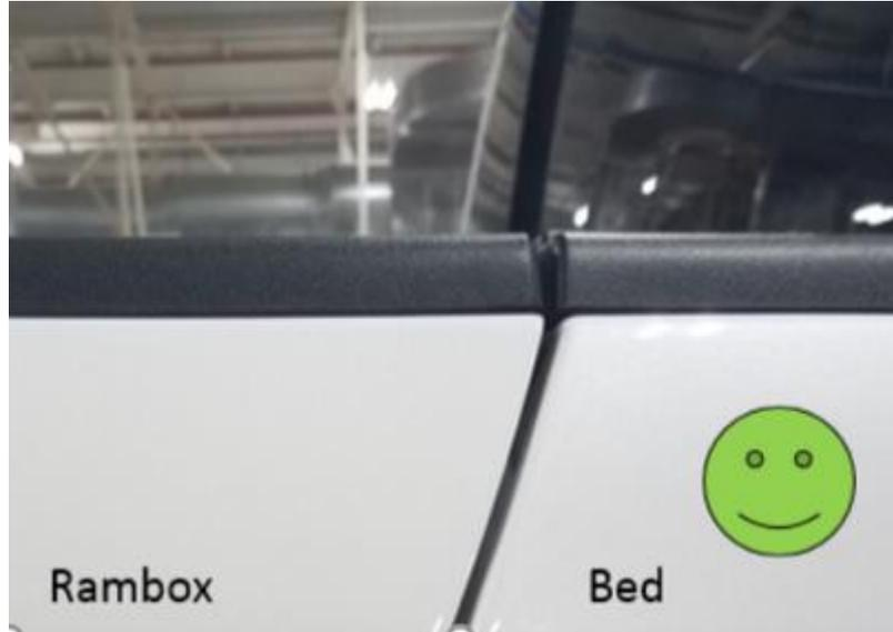
**Verification:** Verify fit and operation. If the RamBox lid (not the applique cover) is warped and the adjustments have not helped, replace the lid with a service part dated after 3/30/2020.
