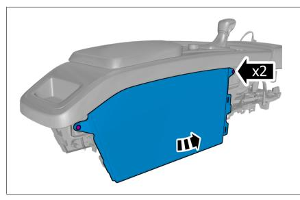
Remove the screws. Remove the marked part.
