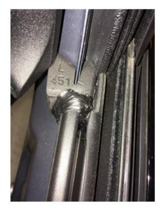
7. Apply the second strip of butyl in a similar orientation to the foam seal at the front of the door (A-Pillar side):
