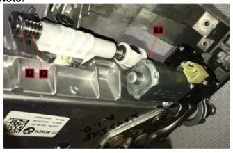
The spindle drive (2) is located on the right side of the steering column as viewed from the driver's seat
