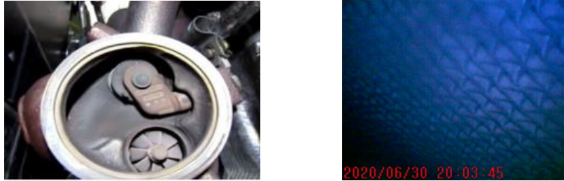
Figure 6: turbo shaft from catalyst side and inside the catalyst
