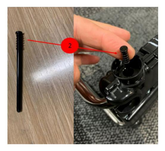
6. Line up the new button assembly key feature with the headrest core key slot (3). Once aligned, install the button onto the new headrest core.
