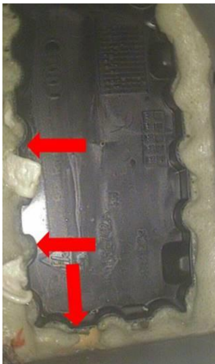
Figure 7. Sound absorber to be completely sealed off.
