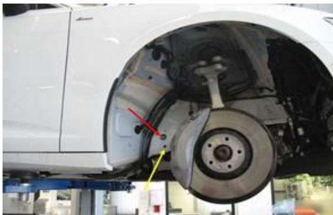
Figure 5. Point of entry for the borescope.
