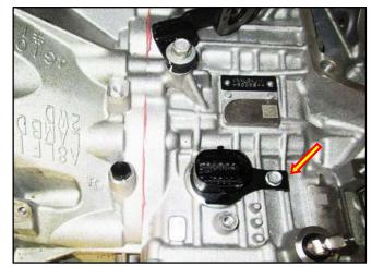
9. Remove 14 oil pan bolts and remove the pan.
