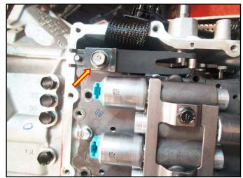
22. Reconnect the harness to the solenoids and install the temperature sensor.
