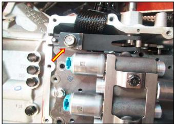
12. Remove 9 valve body bolts in order from the outermost bolts to the innermost bolts.
