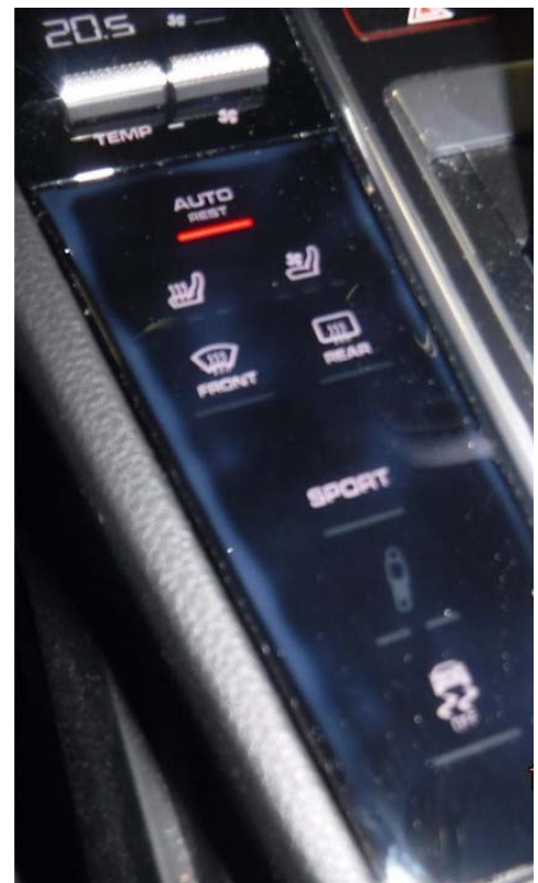
Center console operator control unit discolored at the edges
