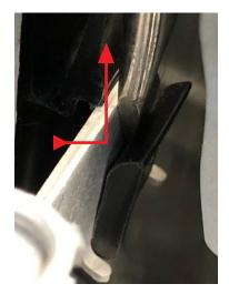
11. Lift the radiator **STRAIGHT UP** only enough to free it from the lower grommets then raise the right (passenger side) of the radiator up APPROXIMATELY 1 INCH which is enough to access the air plug. Remove the air plug using a #2 Phillips screwdriver.
