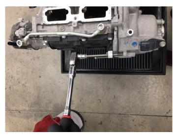
4) CAREFULLY proceed with repeating the Step 3 tightening procedure until there is enough of a gap between the chain cover and the engine for finger access to help with removal. A <u>PLASTIC</u> trim removal too can also be used (especially on the B2 (LH) side as only 1 removal bolt is used). **NEVER** use any metal tools as they can easily scratch / damage the machined mating surfaces.
