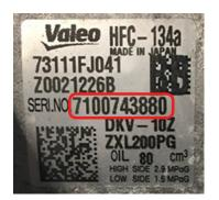
In this example (**710043880**), the "**7**" indicates the production year as 2017 (an "**8**" would be 2018, etc.). The next 2 digits, "**10**" indicates October as the production month (a "**09**" would be September, etc.). **NOTE:** Any compressor with a production date of **810 or HIGHER** (**October 2018 or newer**) had the new valve component installed at manufacture and does <u>NOT</u> require replacement.
