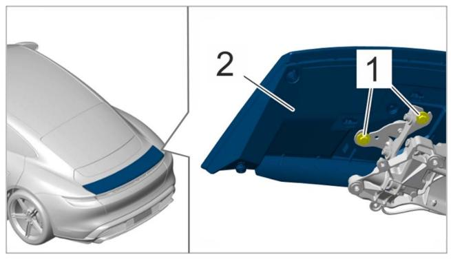
Installation position of screws for rear spoiler blade
