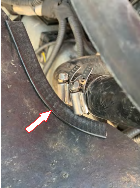
Trim lock installed on splash shield
