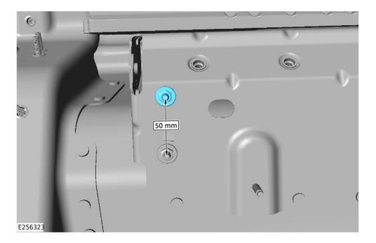
Install a new body ground stud (78905) 50 mm above the existing ground stud (G4D178) (see TOPIx Workshop Manual section 501-25A: Body Repairs General Information - General Procedures - Body Earth Stud Repair).
