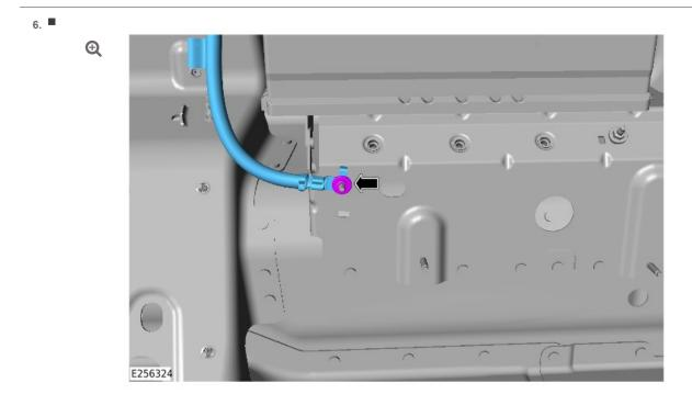
Install the startup battery ground cable to the new body ground stud.
