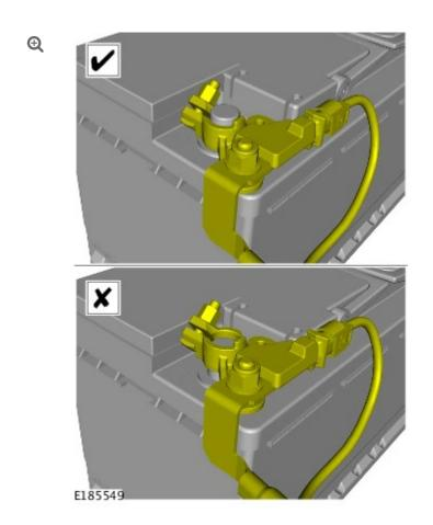
Connect the startup battery ground cable (see TOPIx Workshop Manual section 414-00: Battery and Charging System - General Information - Specifications).
