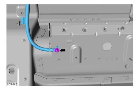
Remove the startup battery ground cable from the body ground stud (G4D178).
