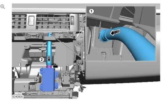
Install the new air ionizer hose.
