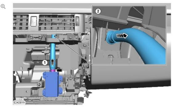
Remove the air ionizer hose.
