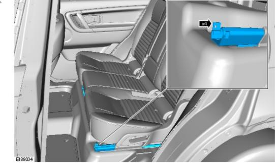
Identify the area of the four second row seat rails to be modified.
