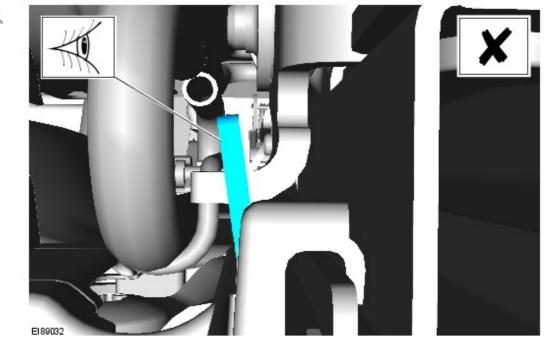
Check the alignment of the seat rail tang.
