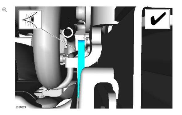
Using a suitable tool, make sure the seat rail tang is in the position shown.
