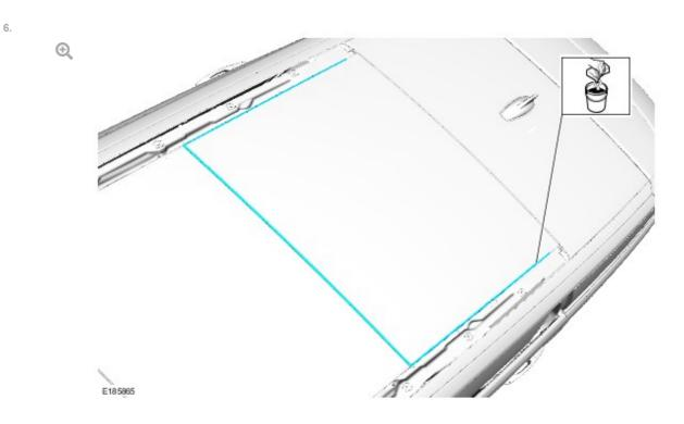
Use a suitable solution (2 ml mild soap per 1 L of water), wet the area shown.
