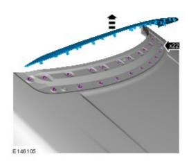
Use a suitable tool to remove the hood finisher.
