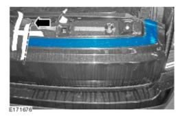
Apply the abrasion protector tape to the vehicle. Make sure the end of the abrasion protector tape is lined up with the masking tape center line.
