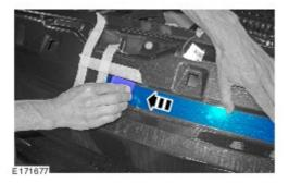
Using a suitable rubber block, smooth the soap/water solution and the air bubbles out from underneath the abrasion protector tape in the direction shown.
