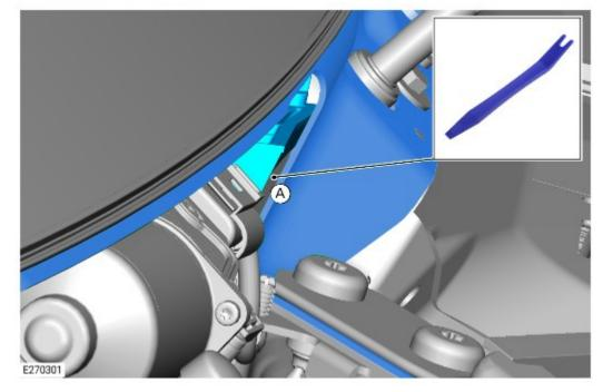
Insert a suitable trim tool between the bulkhead baffle and bulkhead panel (A).
