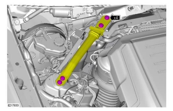
Loosen, but do not fully remove, the support bar retaining bolts.
