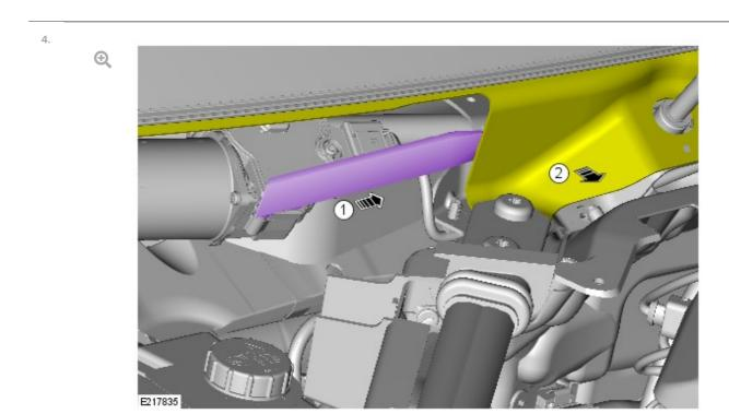
Inserting the suitable trim tool (1) between the bulkhead baffle and bulkhead panel will move the bulkhead panel (2) forward away from the baffle.
