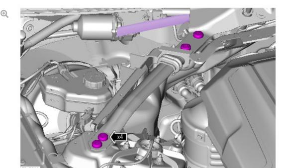
With the trim tool in place, tighten the support bar retaining bolts.
