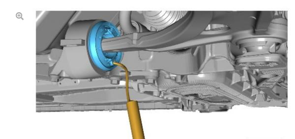
Using a syringe and a length of tube, remove as much hydrabush fluid as possible through the hole created in the fill port. A minimum of **50 ml** of hydrabush fluid must be removed before continuing to step 8.
