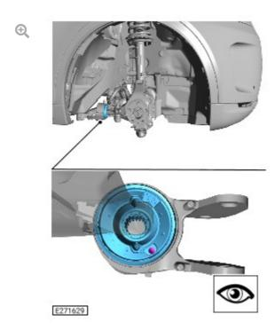
Locate the fill port on the rear hydrabush of the front right lower control arm, as shown in the illustration.
