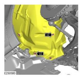
Install front right wheel arch liner in the original position.
