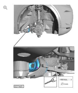
Drill a hole through the back of the hydrabush casing using a 3 mm diameter drill bit, to a depth of no more than 3 mm, this will assist with the removal of the hydrabush fluid in the next step.
