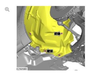
Reposition the front right wheel arch liner.
