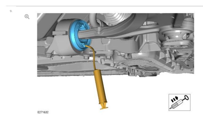
Using a syringe and a length of tube, remove any excess degreaser/hydrabush fluid through the hole created in the fill port.
