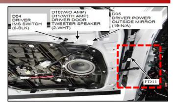
9b. Lift up on the locking tab to disconnect the FD11/FD21 connector.
