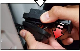
11. Locate the side of the connector with the white locking tab.
