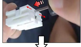
6b. Using a lifting motion, gently pry upwards on each side. The terminal should easily slide out of the back of the connector if done properly.
