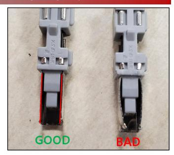
7b. Using needle nose pliers, **gently** squeeze the outer shield on the female terminal to improve the tension. Insert the female pin around the male connector to gauge tension.
