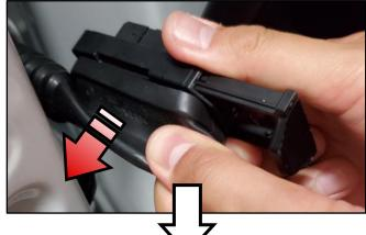
B. Pull the cover down from the connector to expose the wires.
