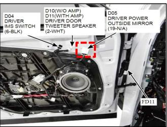
5. Using a pick tool, lift the black locking tab on the two (2) points shown to unlock the wire connectors.
