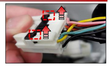
6a. Using a terminal removal tool, work the tool into the hole <u>above</u> the coax terminal in a straight motion.
