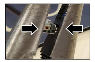
15. Reassemble the coaxial wire in the same reverse order of removal. Ensure the wire is fully seated and the locking tab is secured in place. (Refer to step 11).
