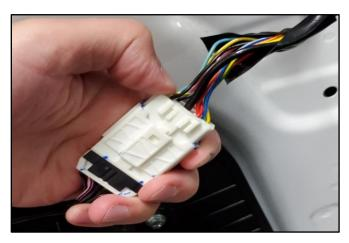
9a. <u>Driver side door</u>: Locate the **FD11** connector in the upper right side of the doorframe. (Refer to image)
