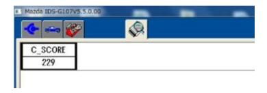
The C\_SCORE indicates the FSC temperature. As the temperature rises, the value of C\_SCORE decreases, therefore "C\_SCORE" must be **174 or higher** to perform the FSC reprogramming.
