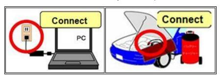
• During reprogramming, connect a battery charger to the vehicle with the charge current maintained within 10 to 15A to stabilize voltage fluctuation.
