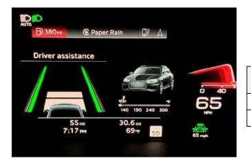
Make sure the update is required by checking • the software version of the installed instrument cluster -J285- (diag. addr. 0017: OBD > 0017 -Instrument Cluster > Identification) against the table below.
